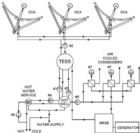
Figure 3 - Process flow diagram for RRES
