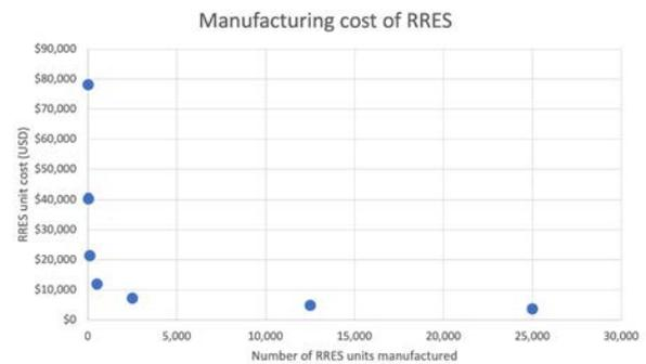
Figure 5 - Relationship of RRES unit cost to manufacturing volume
