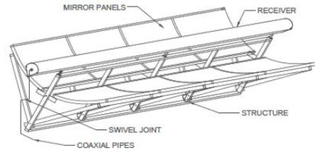
Figure 4 - Detail of the solar collector assembly
